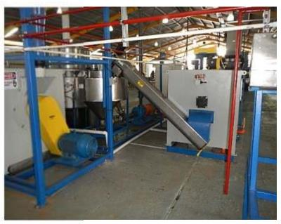
American Cierra Corporation has developed a wash and recycling system that is specifically designed for the Caribbean Islands' recycling program. Although it can be used for any Recycler requiring a small inexpensive recycling plant. The system includes a new High Attrition Washer with Hydro Cyclone Separation, and a Turbo Centrifugal Dryer. This line produces 2,000 lbs. per hour. Other lines can be manufactured to produce much higher rates.
